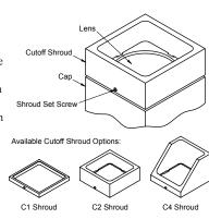
Making sure that the Cutoff Shroud is fully seated on the Cap, slightly tighten the Shroud Set Screw. Note: Do not overtighten set screw. Tighten just enough to secure the shroud.
